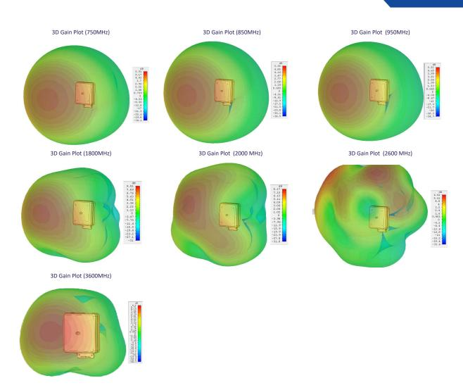
\*WMM8G-7-38 3D Patterns show realised gain both elements fed modelled in CST Microwave Studio without additional cable.
